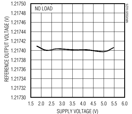
REFERENCE OUTPUT VOLTAGE vs. SUPPLY VOLTAGE
